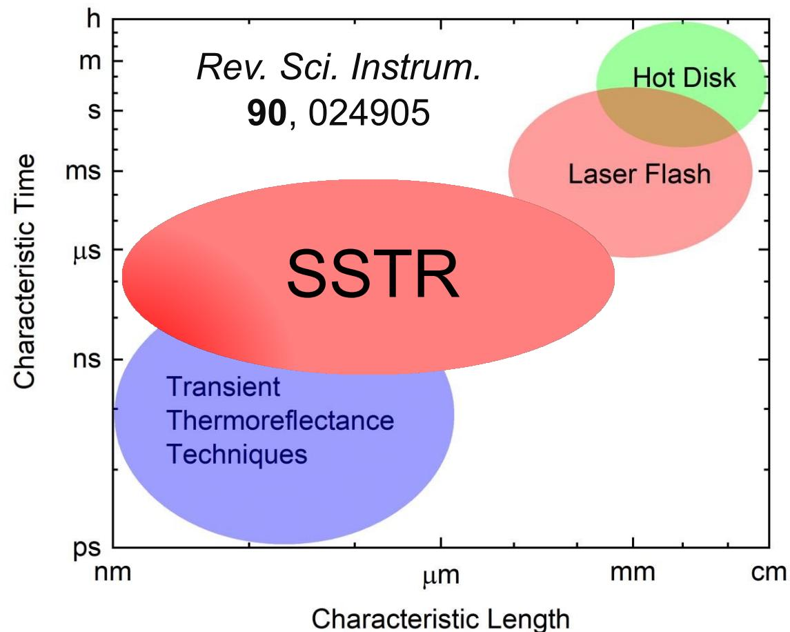
**Spatially resolved thermoreflectance techniques for thermal conductivity measurements from the nanoscale to the mesoscale**
