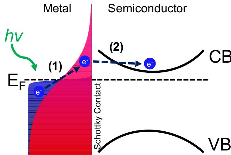
b) Ballistic thermal injection
