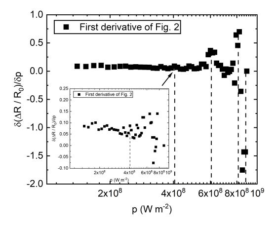
Figure S2. First derivative of our thermoreflectance data shown in Fig. 2 in the main manuscript. The inset shows the critical point near the power density of  $4x10^8$  W m<sup>-2</sup> for clarity.
