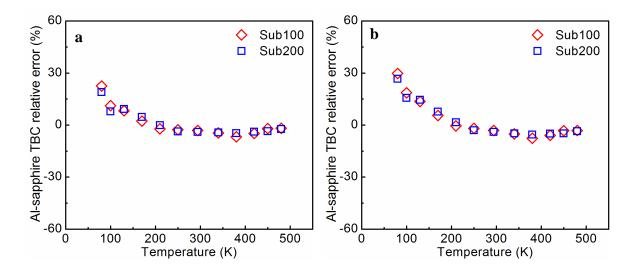
**Supplementary Figure 5**. **a** the relative errors of the measured TBC comparing with the Landauer TBC. **b** the relative errors of the measured TBC comparing with the AGF TBC.
