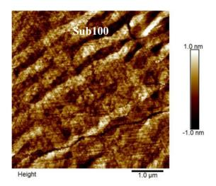
**Supplementary Figure 2**. Atomic Force Microscopy (AFM) images of Al surface. Root-mean-square (RMS) roughness for a 5  $\mu$ m x 5  $\mu$ m area is 0.288 nm for Sub100. The scale bar is 1 um.
