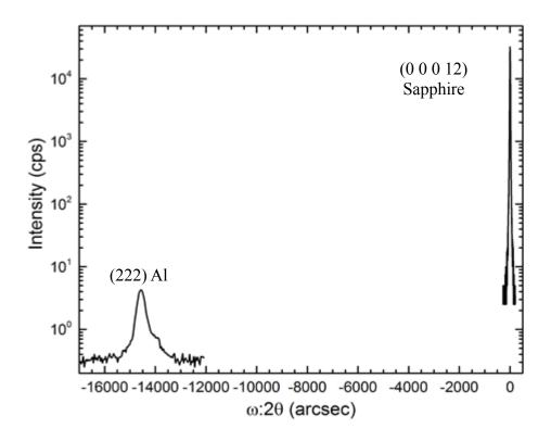
**Supplementary Figure 4**. Triple-axis diffraction results of Sub100. The experimental conditions of triple-axis diffraction on Sub100 are, detector slits: 1375" divergence, Al FWHM: 251", Step: 30", Count: 360 sec. The (222) Al is -14565" away from the (00012) Al<sub>2</sub>O<sub>3</sub> peak so the experimental  $a(Al) = 4.0422 \pm 0.0007$  Å while an Al powder measurement using the same equipment is  $4.04236 \pm 0.00009$  Å. Therefore, Al film in Sub 100 (and Sub 200) is strain-free.
