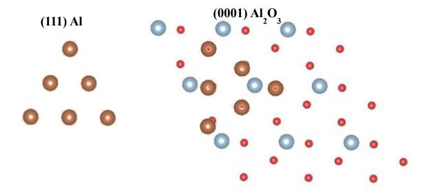
**Supplementary Figure 1**. Schematic diagram of crystal structure of Al and sapphire. For (111) Al, distance between adjacent Al atoms =  $d_{[\underline{1}10]} = 2.863583$  Å. Distance between adjacent O atoms =  $(2/3)d_{[\underline{1}0\underline{1}0]} = 2.747733$  Å. The mismatch is ~4% if the Al metal aligns with the O from sapphire. Note that images are to scale and color difference is to show clarity between Al from metal and sapphire.
