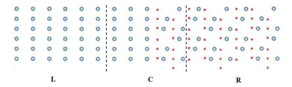
**Supplementary Figure 6**. Schematic of the Al-sapphire system. L, C and R mean left lead, central region and right lead, respectively.
