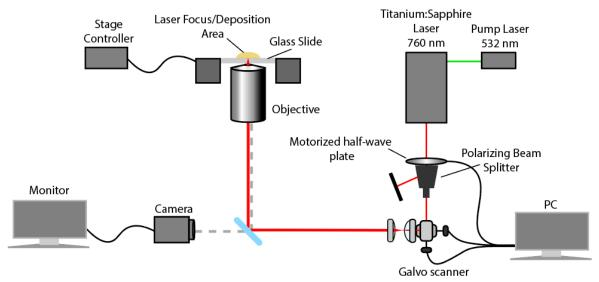
**Scheme S1.** Schematic representation of the direct laser writing optical setup, as described in detail in the Supporting Information section "Direct Laser Writing Optical Setup".
