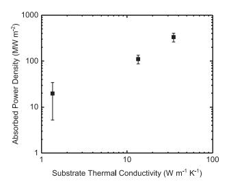
FIG. 2. Measured absorbed power density necessary to form Ag microstructures on substrates (i.e., power threshold necessary to induce direct write) as a function of thermal conductivity of the substrate using a continuous wave, 532 nm beam.
