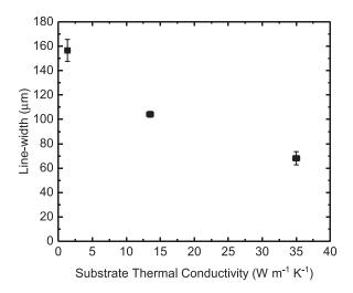
FIG. 1. Measured line-width for Ag microstructures at an absorbed power density of  $\sim 350\,\text{MW m}^{-2}$  for substrates of varying substrate thermal conductivity; these were synthesized with a CW 532 nm beam.
