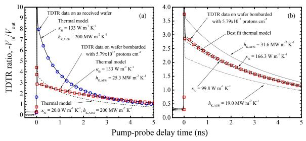
FIG. 1. (Color online) (a) Example of model fit to TDTR data on the as received Al/Si sample, and the Al/Si sample in which the Si substrate was subjected to ion dose of  $5.79 \times 10^{17}$  protons cm<sup>-2</sup>. In the proton irradiated case, the model achieves a best fit to the data by only adjusting  $h_{\rm K}$ . Adjusting  $\kappa$  results in a poor fit. (b) Sensitivity of the best fit model on the proton irradiated data in (a) to a  $\pm 25\%$  change in  $\kappa$  or  $h_{\rm K}$ .
