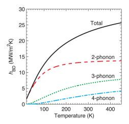
Fig. 1 Individual contributions of two-, three-, and fourphonon processes for Au to c-axis graphite thermal boundary conductance
