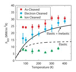
Fig. 3 Measured thermal boundary conductance as a function of temperature for various surface preparations of Au-HOPG compared to the elastic and inelastic modified DMM models
