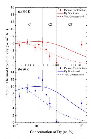
FIG. 3. Phonon thermal conductivity of CdO:Dy at (a)  $300\,\mathrm{K}$  and (b)  $80\,\mathrm{K}$  along with bounding models for a system dominated by scattering from Dy doping (solid lines: "Dy Dominated") and a model for a system with additional scattering from vacancies with concentrations pinned by the Dy concentration (dashed lines: "Vac. Compensated").
