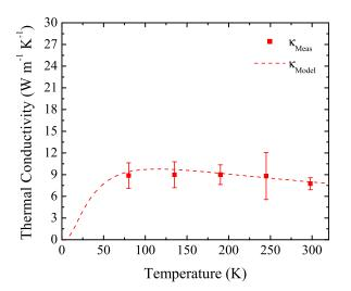
FIG. 2. Measured thermal conductivity as a function of temperature of the undoped film for calibration of the model of thermal conductivity of CdO thin films (dashed line).
