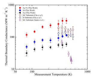
FIG. 2. Thermal boundary conductance as a function of temperature across the metal-GaN interfaces measured in this study (solid symbols) and various GaN-substrate samples from previous literature (GaN-SiC: Cho *et al.*, <sup>34</sup> GaN-Si: Cho *et al.*, <sup>34</sup> GaN-SiC: Sarua *et al.* <sup>4</sup>).
