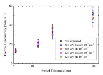
FIG. 4. Thermal conductivity of Cu–Nb multilayers plotted versus period thickness. The figure shows that ion irradiation of different energies and doses of helium ions or protons does not affect the magnitudes of thermal conductivity of Cu–Nb multilayers. This demonstrates the possibility of using Cu–Nb multilayers as radiation resistant materials in advanced nuclear systems.
