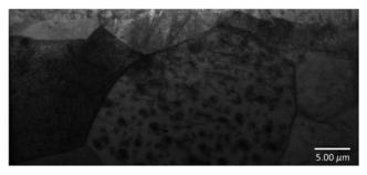
FIG. 3. Cross-sectional TEM (Ref. 50) on optimized ZIRLO showing the variation in the microstructure.
