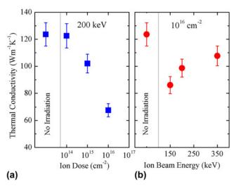
FIG. 5. Thermal conductivity of silicon plotted as a function of (a) proton irradiation dose at a constant beam energy of 200 keV and (b) proton beam energy at a constant dose of  $10^{16}$  cm<sup>-2</sup>. The data indicate a drastic reduction in thermal conductivity with dose as compared to the nonirradiated sample and an increase in thermal conductivity with ion beam energy.
