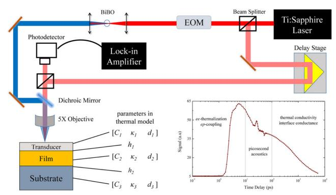
FIG. 1. A simplified schematic of the main components of our TDTR system. In the thermal model, each layer is represented with three parameters: the volumetric heat capacity, C, the thermal conductivity,  $\kappa$ , and the thickness, d. The figure also shows a plot of a typical TDTR measurement. The plot was shifted by +7 ps to allow for logarithmic scaling.
