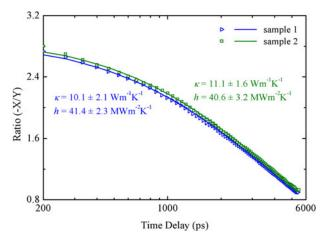
FIG. 2. Data points (symbols) and best fit curves (solid lines) for the TDTR measurements on Al/optimized ZIRLO samples 1 and 2. The average thermal conductivity of optimized ZIRLO from the two measured samples is 10.7  $\pm$  1.8 W  $m^{-1}\ K^{-1}$  as determined from our multiple TDTR measurements.
